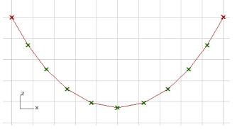
a flexible cable is modelled as made up of multiple straight segments
