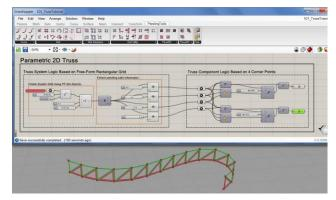
2- To define the system logic, first we need to create a grid. In this case our grid is based on a curve<sup>1</sup>. First step is to create a reference a curve in Rhino, then divide the curve by distance which represents the width of the truss.
