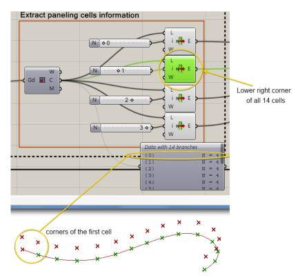
6- Create custom component logic that is based on 4 corners and feed system grid or cells corners into the component logic.
