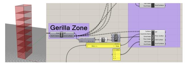
Above we are assigning a wall assembly to every wall surface using the Series component we used previously and selecting Wall Index 1,2,3, and 4 using a panel.
