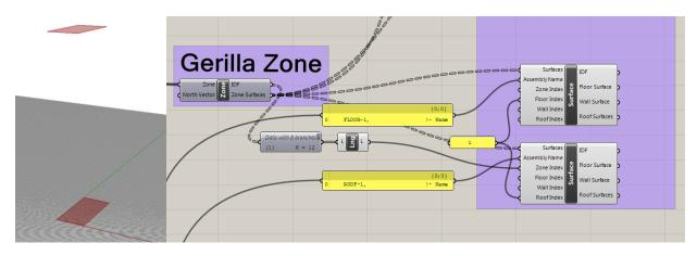
Above we are assigning a floor assembly to the floor of the first zone and a roof assembly to the roof of the last zone selected using a list length component.
