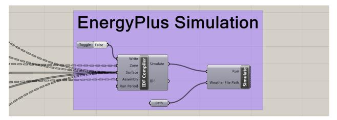
The Gerilla Zone component IDF attaches to the IDF Compiler Zone input. All of the Gerilla Surface IDF's connect to the Surface input. Connect the Gerilla Assembly Component IDF to the Assembly input for the IDF Compiler component. The default Run Period is all year, so we don't need to plug anything in here. Attach a Boolean to the Write input for IDF Compiler component.
