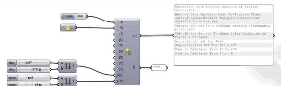
Calculates incident solar radiation levels (insolation) over the current analysis grid or objects within the model
