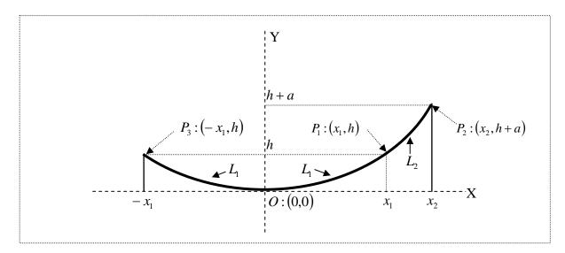
In the drawing above you can see a rope fixed at 2 ends  $p_3$  and  $p_2$  with different heights. In this drawing h represents the height of  $p_3$  above the lowest point of the curve. If we call d the horizontal distance between points  $p_3$  and  $p_2$  you can see that  $d = x_1 + x_2$  and if the total length of the rope is called L it follows that  $L = L_2 + 2L_1$ . Also a is the height difference between the points.
