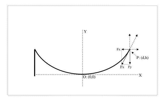
The aim of this document is to determine which function describes the curve of a rope hanging (in a steady state) between two fixed points. In order to make this possible we need to assume a few things about the rope.
