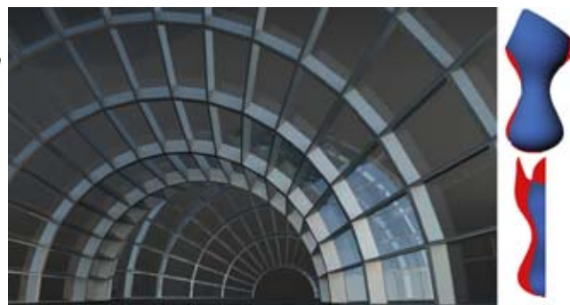
Figure 5: A rotational surface with PQ panels compared with original surface
