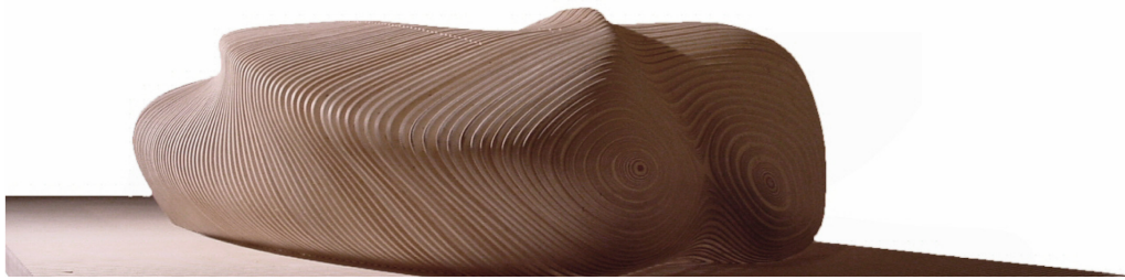
Figure 2. The prototype produced by five axes CNC milling (Photo: courtesy of dECOi Architects).
